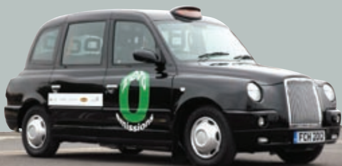
The hydrogen fuel cell taxi produced by Intelligent Energy.
