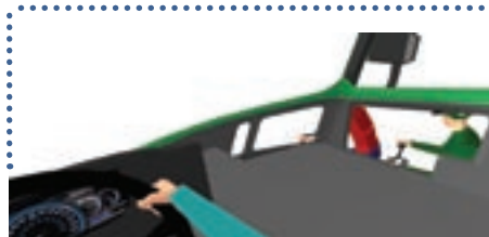
The Direct Vision concept aims to reduce the driver's reliance on mirrors, in favour of greater direct visibility and fewer blind spots.
