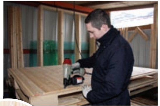
● Far left: Steve Clear; left and above: containers are made from 8mm Scandinavian redwood tongue and groove in the company's workshops.
