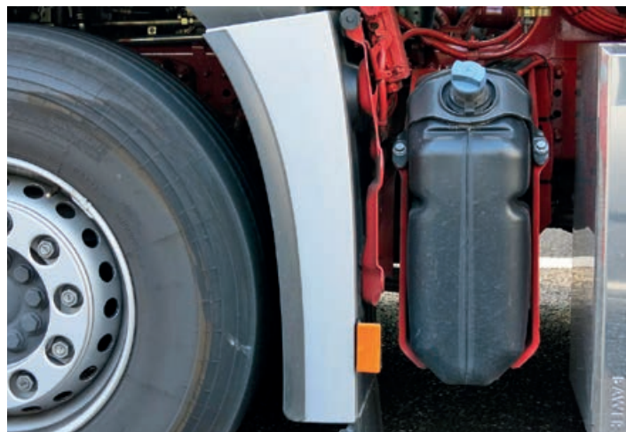
● AdBlue is carried in a tank fitted to the vehicle.
