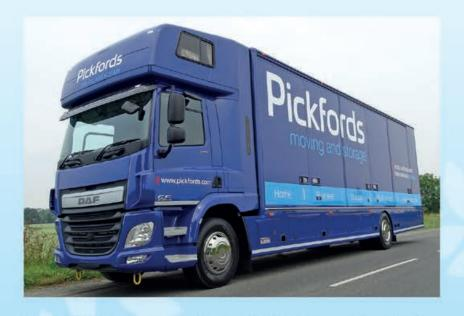
New DAF CF sleeper cab, fitted with five container body and Supremacy double sleeper pod.
