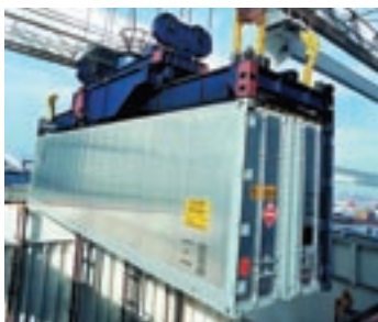
● Verifying the container's weight on the loading crane is too late as the loading position has already been determined.
