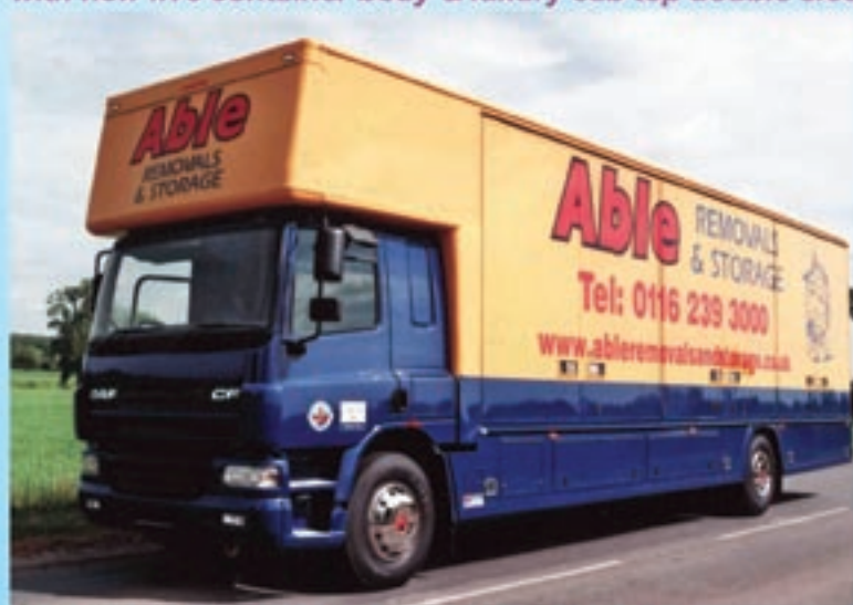
Fully refurbished DAF 65 series chassis with sleeper cab, fitted with new six container luton body.
