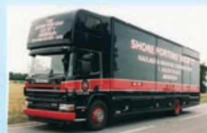
Fully refurbished DAF 65 series chassis with sleeper cab, fitted with new five container body & luxury cab top double sleeper pod.
