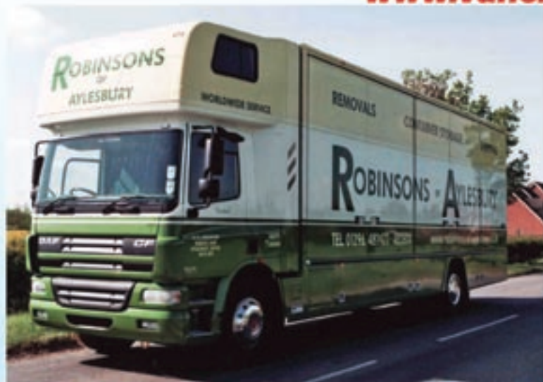
Fully refurbished DAF 65 series chassis with sleeper cab, fitted with new five container body & luxury cab top double sleeper pod.
