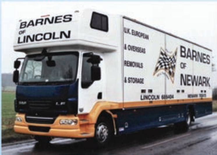
Six container body, with luxury cab top double sleeper pod, fitted to a new DAF 55 series chassis with sleeper cab.
