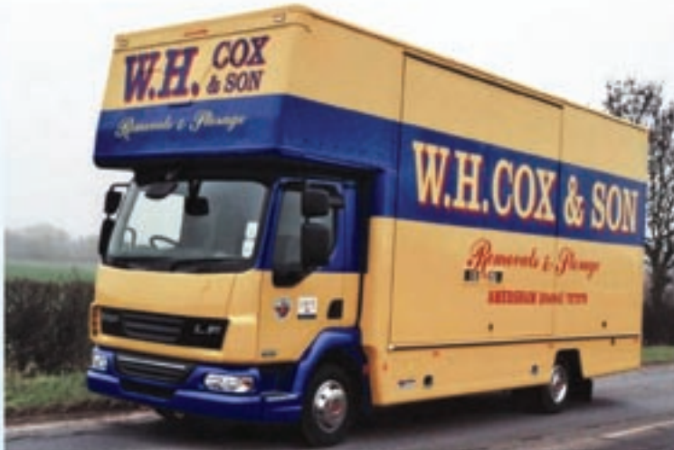
Three container body, fitted to a fully refurbished DAF 45 series chassis.
