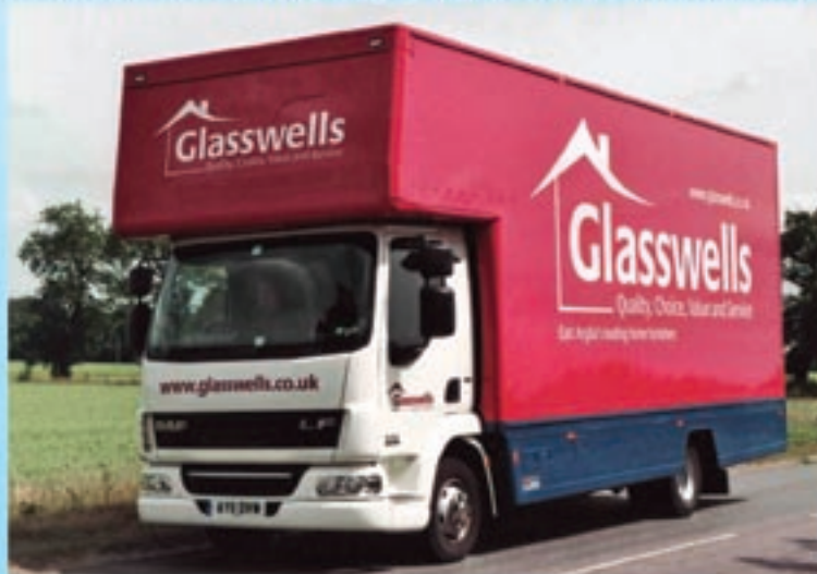
New DAF chassis, fitted with 1,450 cu.ft. luton body.
