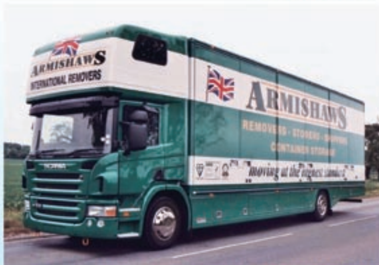
New Scania chassis, fitted with six container drawbar specification body, and luxury cab top double sleeper pod.
