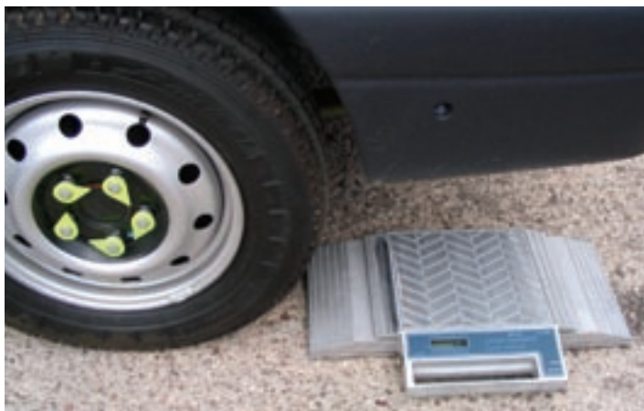
● A vehicle about to be weighed on Red Forge's Axalert Plus display.
