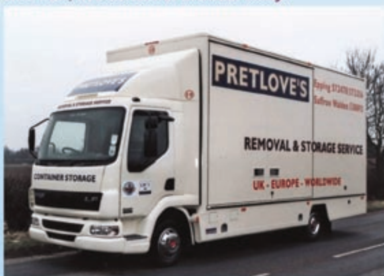
Fully refurbished DAF 45 series chassis/cab, fitted with full air management kit, and new three container body.
