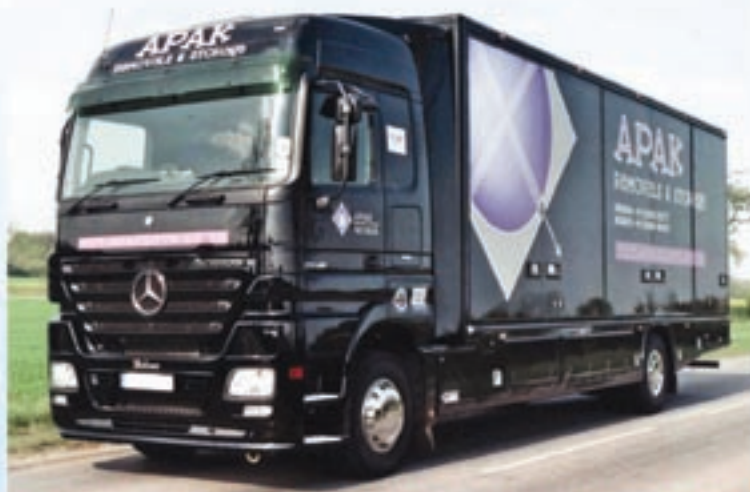
Fully refurbished Mercedes Megaspacer chassis, fitted with new, five container drawbar body.
