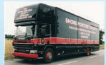
Fully refurbished DAF, fitted with three container bodywork, and air management equipment.
