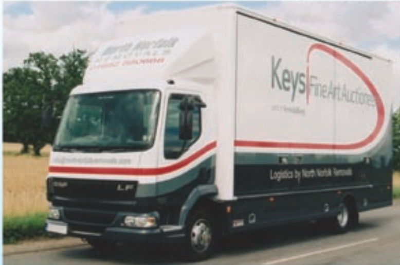
Fully refurbished DAF, fitted with three container bodywork, and air management equipment.
